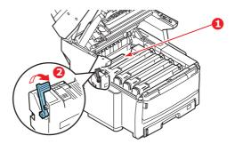
**6.** Holding the fuser by its handle (1), lift the fuser straight up and out of the MFP. If the fuser is still warm, place it on a flat surface which will not be damaged by heat.
